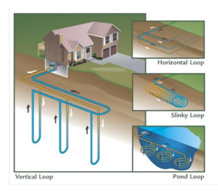
Figure 28 . Different types of Ground Source Heat Pumps (Source: <u>http://www.puregreenenergy.co.uk/Products/DrillingAndTrenches.html</u>)
