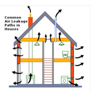
Figure 15. Common air leakage paths (Source: <u>http://www.airtightbuilding.com/</u>)
