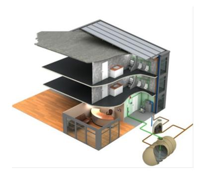
Figure 17. Typical commercial rainwater harvesting system (Source: <u>http://www.kingspanwater.com/</u>)
