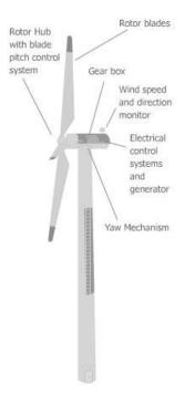
Figure 26 . A typical large turbine (Image courtesy of RenewableUK)
