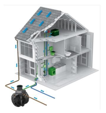
Figure 16. Typical residential rainwater harvesting system (Source: <u>http://www.kingspanwater.com/</u>)
