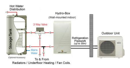
Figure 29 . Air-to-water system (Source: <u>www.thefueleffect.co.uk/Default.asp?Page=19</u>)
