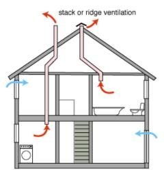
Figure 11. Passive stack ventilation (Source: www.greenspec.co.uk/whole-house-ventilation.php)
