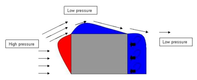
Figure 10. Wind driven ventilation
