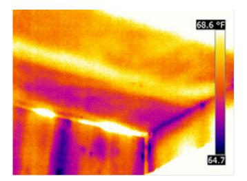
Figure 14. Thermal image showing thermal bridges at the junctions of walls and floors (Source: <u>http://www.flickr.com/photos/pcw\_1333/4457268155/in/photostream</u>)
