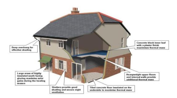
Figure 9 . Exploiting thermal mass on a year-round basis (Source: www.sustainableconcrete.org.uk/sustainable\_design\_constructio/thermal\_mass.aspx)
